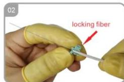
Press the cable into the clamp.
