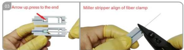
Press the cable into the clamp
